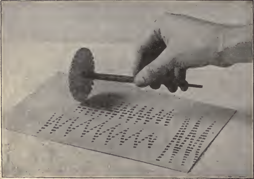
FIG. 43—The roulette (restored) inked and rocked on a sheet of paper.
