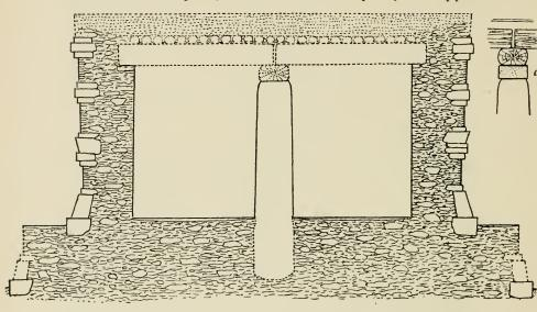
TRANSVERSE SECTION OF BUILDING OF DOUBLE BEAM SPAN.\*
